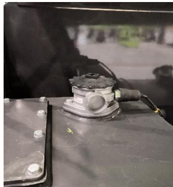
Figure 5-4 Hydraulic return filter
