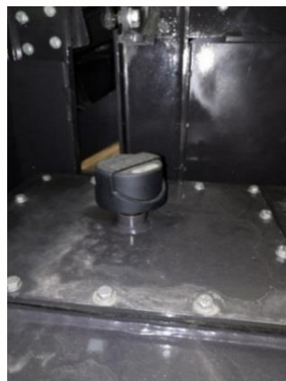
Figure 5-5 Hydraulic Tank Breather
