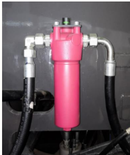
Figure 5-11 High pressure filter
