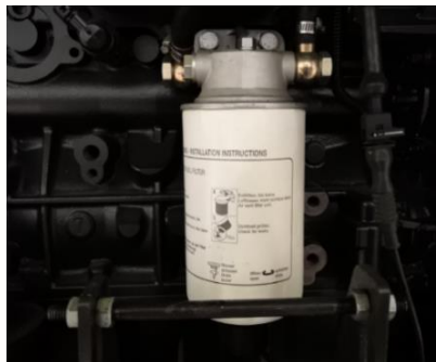
Figure 5-9 Second class fuel filter
