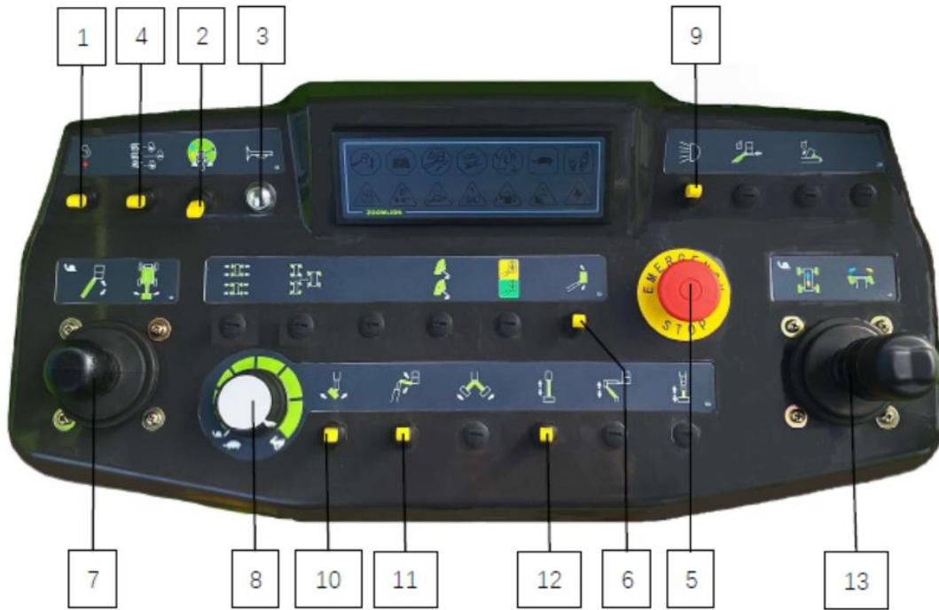
Figure 2-12 Platform Control Panel
