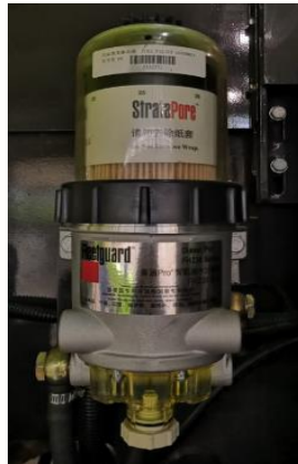
Figure 5-8 First class fuel filter
